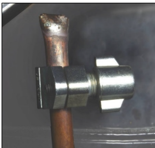
Figure I-3. Piercing-type access valve on a small appliance with nonflammable refrigerant
