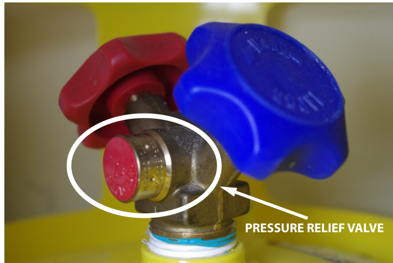
Figure C-9. Pressure relief valve on a recovery cylinder
