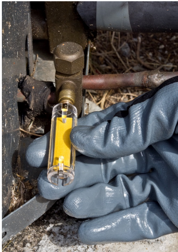
Figure C-11. QwikCheck ® testing for acid on an operating system
