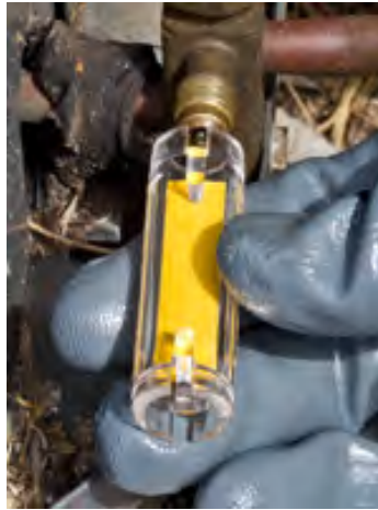
Figure 13. QwikCheck® is yellow before acid test.
