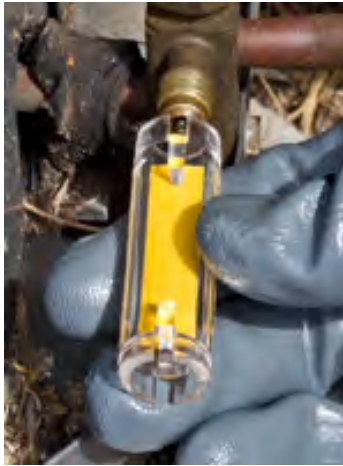
Figure 3. QwikCheck® before acid test
