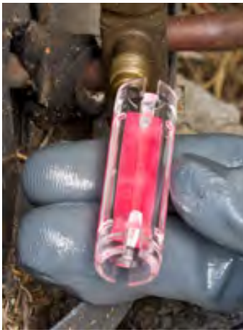
Figure 4. QwikCheck® after acid test if acid is present
