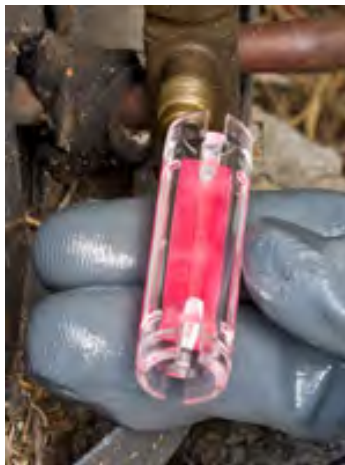
Figure 14. QwikCheck® is orange to red after acid test if acid is present.
