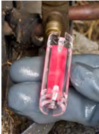
Figure 15. Red QwikCheck® indicates acid is present.
