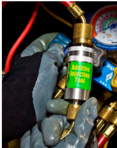
Figure 18. QwikShot® injected into system using QwikInjector®
