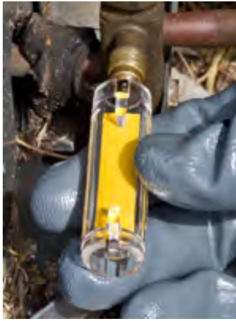
Figure 16. Yellow QwikCheck® indicates no acid is present.
