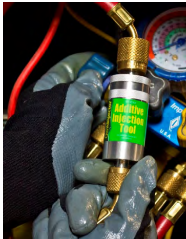
Figure 6. QwikInjector® connected inline for use
