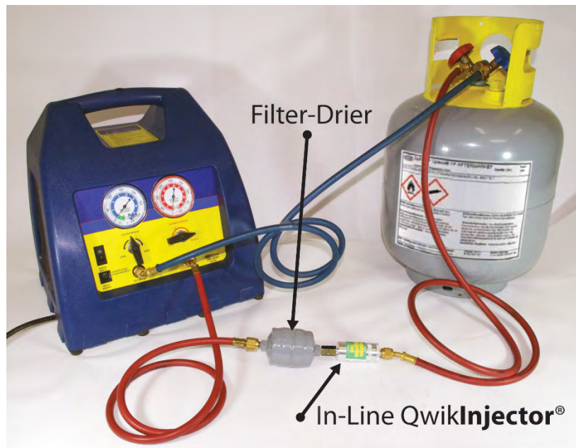
Figure 7. Photo of refrigerant being cleaned and filtered
